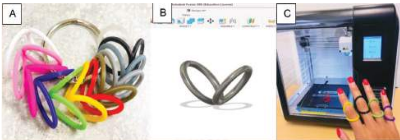
Figure 1. (A) 12 color palette for customization, (B) Orthotic design via Autodesk Fusion 360, (C) Multicolored orthoses and Adventurer 3 3D-printer used.
