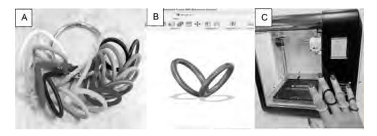
*Figure 1. (A)* 12 color palette for customization, *(B)* Orthotic design via Autodesk Fusion 360, *(C)* Multicolored orthoses and Adventurer 3 3D-printer used.
