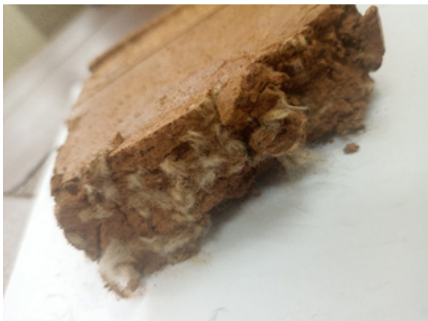
Figure 1 : Laterite cement composite with cotton wastes fibres
