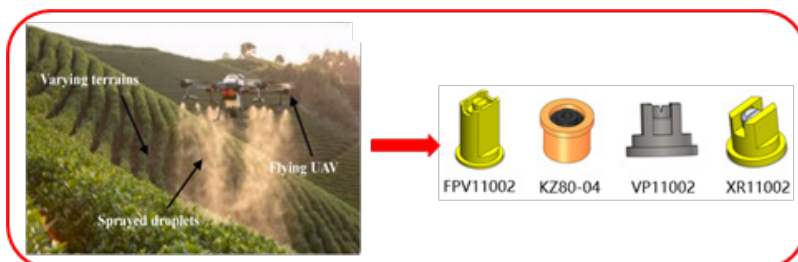
Fig. 1. Six-rotor UAV based spray under different nozzle categories in the Chinese tea plantation
