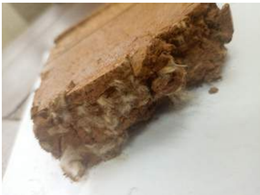
Figure 1 : Laterite cement composite with cotton wastes fibres
