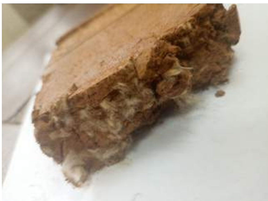
Figure 1 : Laterite cement composite with cotton wastes fibres
