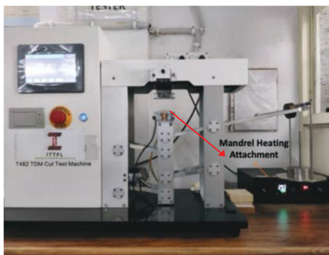
Figure 1 Modified TDM Cut Testing Machine
