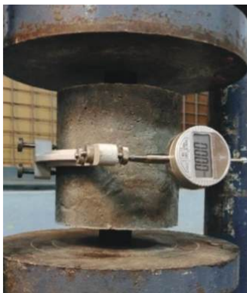
Fig: Double punch test setup
