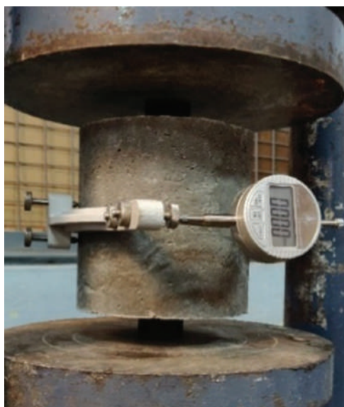
Fig: Double punch test setup
